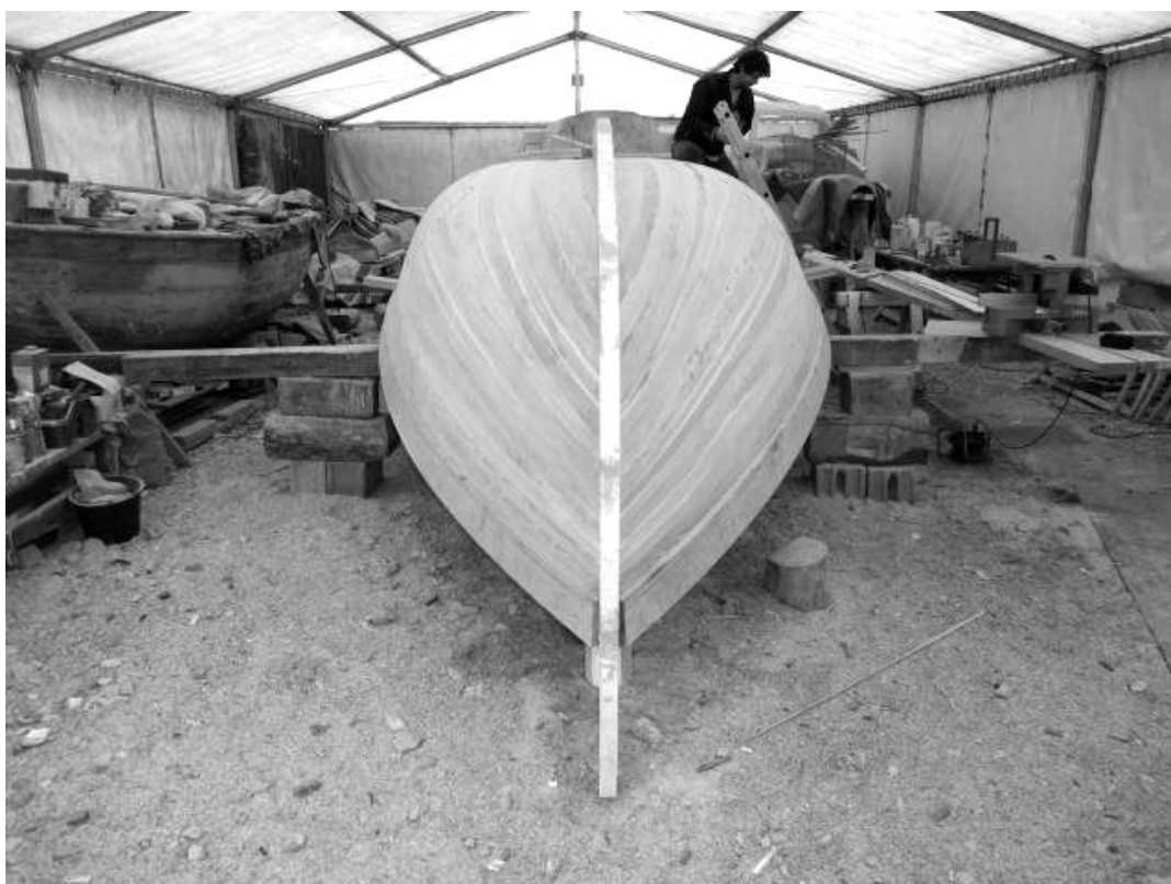
Photo 9: Gajeta falkuša built using cold molded lamination techniques (photo: http://www.betinskagajeta1740.hr )
